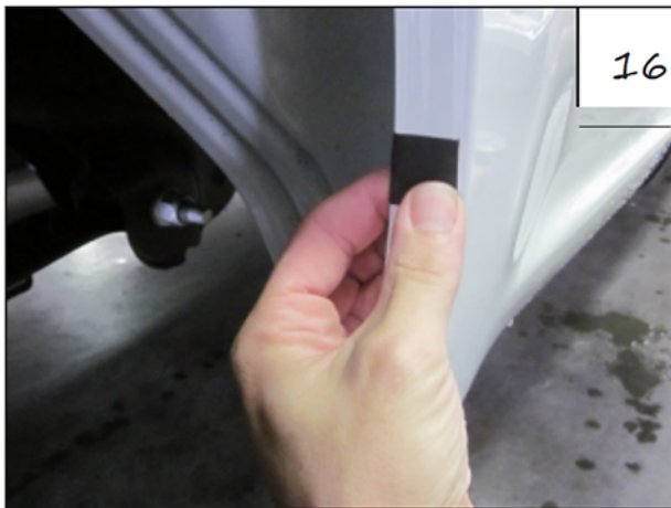
Wrap a MylarTab (MT1-0014) around the wheel well sheet metal, centered over each of the three marks made in Step 15.
