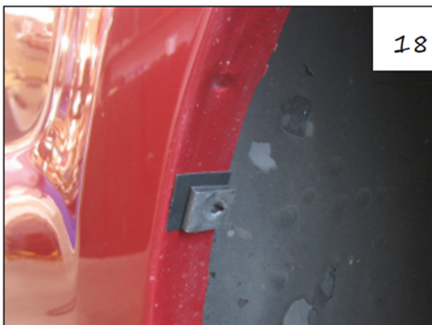
Install a Clip (CL1-0005) over each of the three Tabs (MT1-0014) placed over the upper 3 marks made in Step 16.
