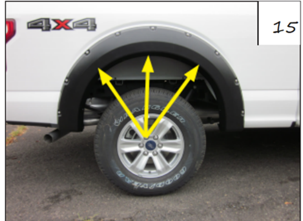
Hold flare to vehicle and mark three flare hole locations with a grease pencil.
