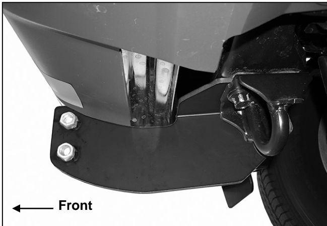
(Fig 8B) Install Frame Bracket with factory tow hook bolts. Small tow hook pictured FOR EXAMPLE ONLY
