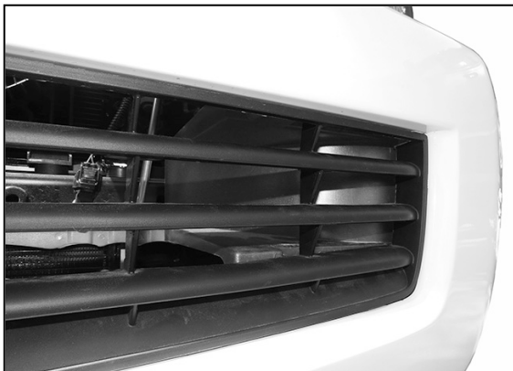
(Fig 5A) Remove or cut air deflector from behind lower grille opening in bumper
