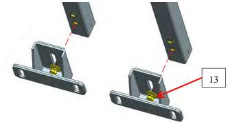
Step 3: Next, place the installed tire carrier assembly (1) in the appropriate position on the trunk, and mark the mounting points of the Connecting Plates (2). Drill a hole with a diameter of 13.8 on the trunk, then install the rivet nut M10\_18 (9) onto the trunk.
