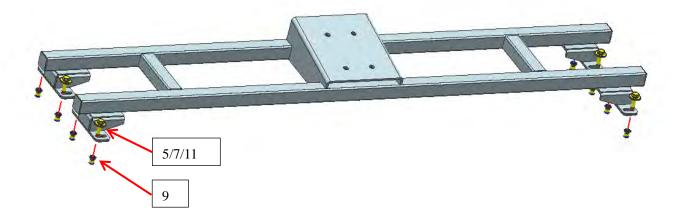
Step 5: Final use the standard parts (6/8/12) to install Universal Lug Plate (3) on tire carrier assembly (1).
