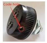
Remove the coding pin to lock in the combination. Test the lock operation before closing the safe door. Please note: The combination can only be changed again by setting the saved combination and inserting the pin. Please record the combination on the card provided.
