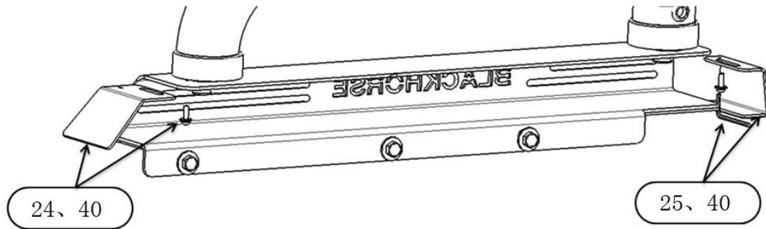
**Notice:** If compatible with tonneau cover, pls sticker the black adhesive tape 21 on the truck rail to full fill the gap as the picture shown.
