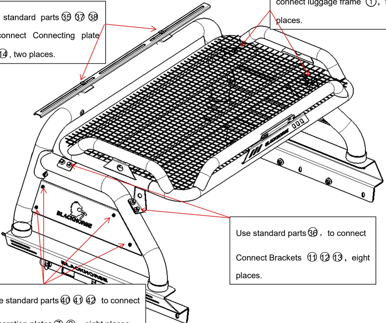
**Step3:** Put roll bar on the truck in an appropriate place. And use pen to mark the holes. 3 places in each part, 6 places total. Remove the roll bar then drill the size of  $\Phi 12$  holes. Put the roll bar back and use standard 30
