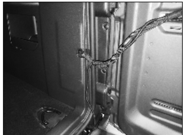
(Fig 16) Run the License Plate Harness up from behind Bumper, over the door seal and up to the factory harness.
