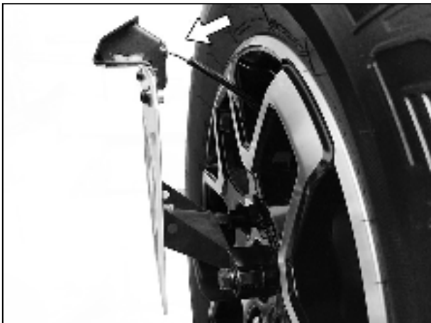
(Fig 20) Plug Harness into license plate light
