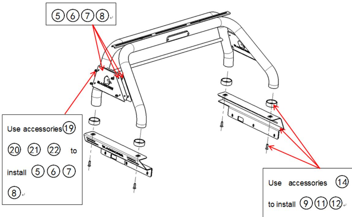
**Step 3:** Connect brackets and roll bar with standard parts as figure shows.
