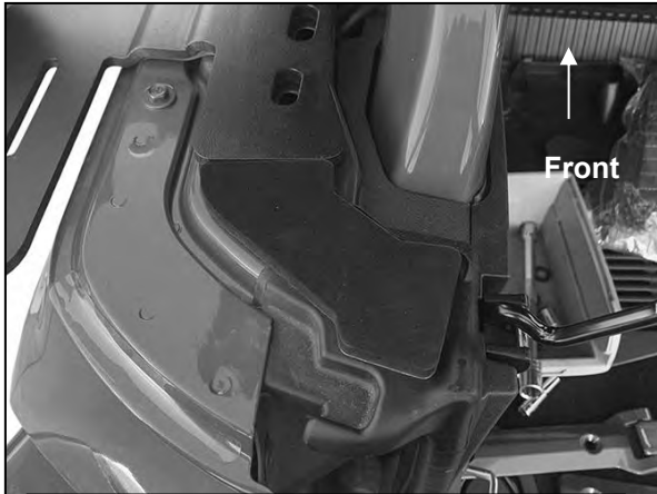
(Fig 13) With Front Spacer, Seals and Bracket in place, reinstall top (driver/left side pictured)
