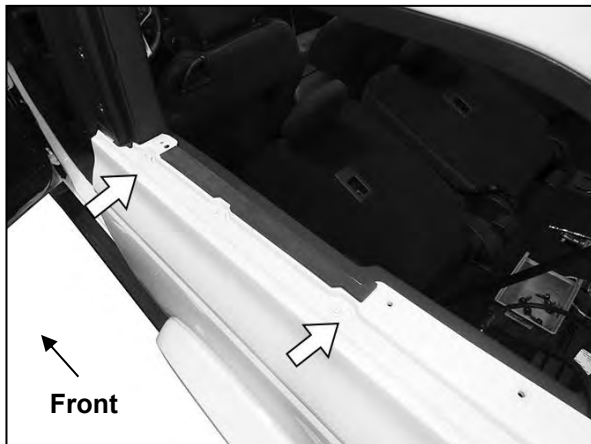
(Fig 11) Remove backing and apply driver/left adhesive backed Foam Side Seal to top of body (arrows)
