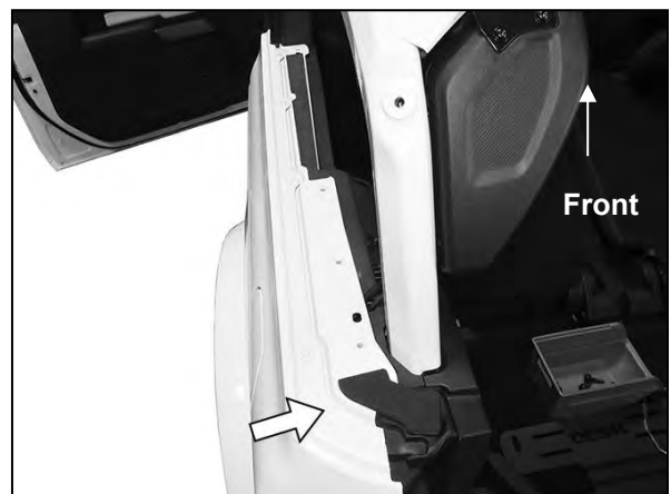
(Fig 12) Apply adhesive backed Foam Rear Seal to top of body
