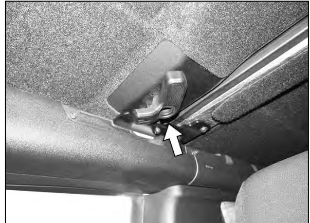
(Fig 18) If necessary, loosen screw 2-3 turns to adjust and fasten latch (arrow)
