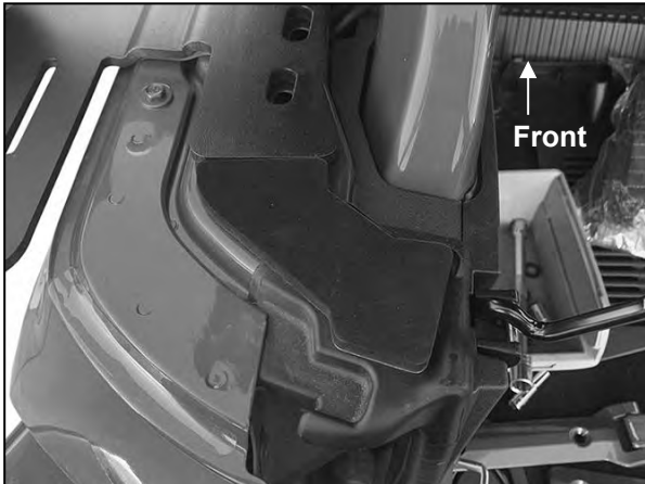
(Fig 21) Apply adhesive backed Foam Rear Seal to top of body, between top frame and body (driver/left side pictured)
