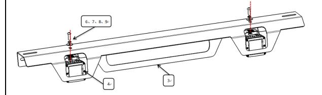
**Step2:** Install (1)(2)(3) and (4) with (6)(7)(8)(9) as below diagram shows.
