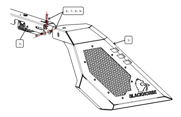
Step 3: Connect brackets and roll bar with standard parts 16 18 19 20 as figure shows.
