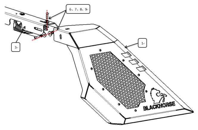
Step 3: Place the brackets on the truck. Drill the  $\Phi$  12 size of holes for installing backets.
