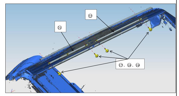
Step 4: Connect brackets and roll bar with standard parts 1 (1) (1) (1) as figure shows.
