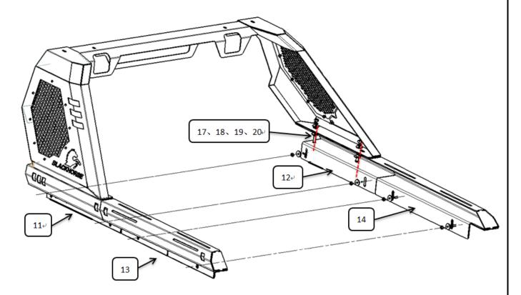
Step 4: Test and make sure that the roll bar is steadily fixed, fully tighten all hardware.
