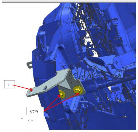
Step 4: Fix driver/left support bracket 2 with standard parts and support bracket 1, consistent on both sides, the following figure shows the left side.
