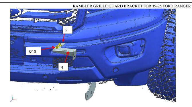
Step 5: Use standard parts to fix the driver/left mounting bracket, driver/left support bracket 2 and bumper, with consistency on both sides, the following figure shows the left side.
