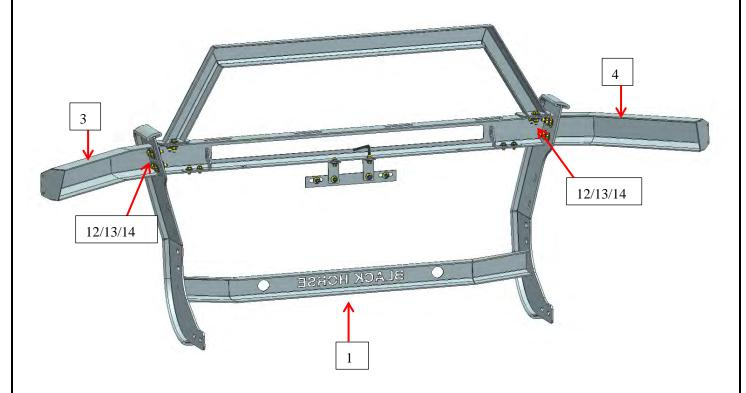
Step 6: Find 2 radar holes on the grille guard and install them according to the standard parts shown in below pictures.
