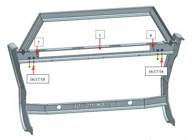
Step 4: Use standard parts to install License Brackets 1 and 2 with Main Guard as below figure shown.
