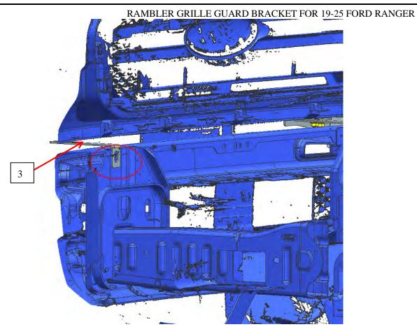
Step 3: Find the installation hole for the driver/left mounting bracket of the vehicle code on the body beam, and fix it to the beam using standard parts 6/7/9, consistent on both sides, the following figure shows the left side.
