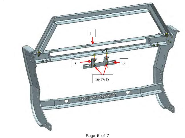
Step 5: Use standard parts to install Left and Right Side Bars with Main Guard as below figure shown.
