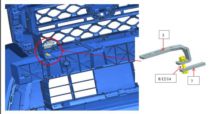
Step 3: Find the installation hole for the driver/left mounting bracket of the vehicle code on the body beam, and fix it to the beam using standard parts 9/11/15, consistent on both sides, the following figure shows the left side.
