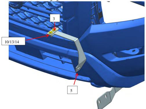
Step 5: Use standard parts to fix the driver/left mounting bracket, driver/left support bracket 2 and bumper, with consistency on both sides, the following figure shows the left side.
