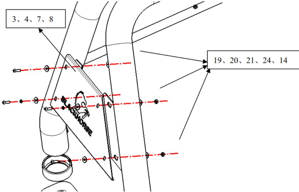
Step 4: Using wrench 13, install support plate 10 and gum cover 9 with part 26.
