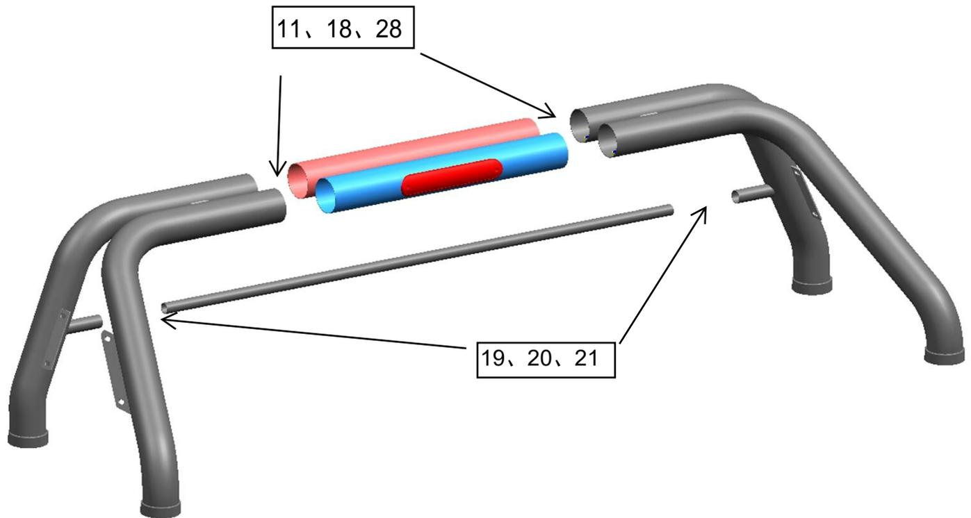
Step 2: Using wrench 15, install 1/2 main pipes and connecting plate 5 together with parts 9/10/11/13 as shown.
