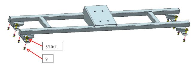
Step 5: Final use the standard parts (4/5/7) to install Universal Lug Plate (2) on tire carrier assembly (1).
