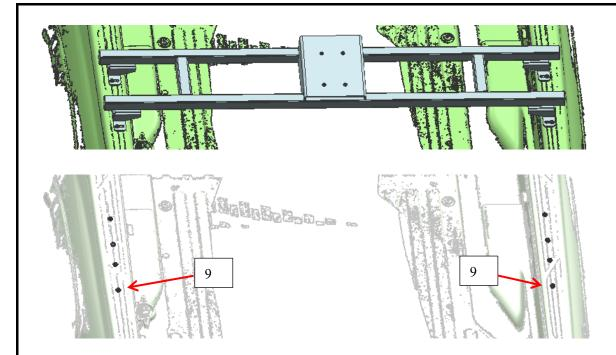
Step 4: Use standard parts (8/10/11) to install the tire carrier assembly (1) onto the trunk.
