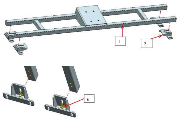
Step 3: Next, place the installed tire carrier assembly (1) in the appropriate position on the trunk, and mark the mounting points of the Connecting Plates (3). Drill a hole with a diameter of 13.8 on the trunk, then install the rivet nut M10\_18 (9) onto the trunk.
