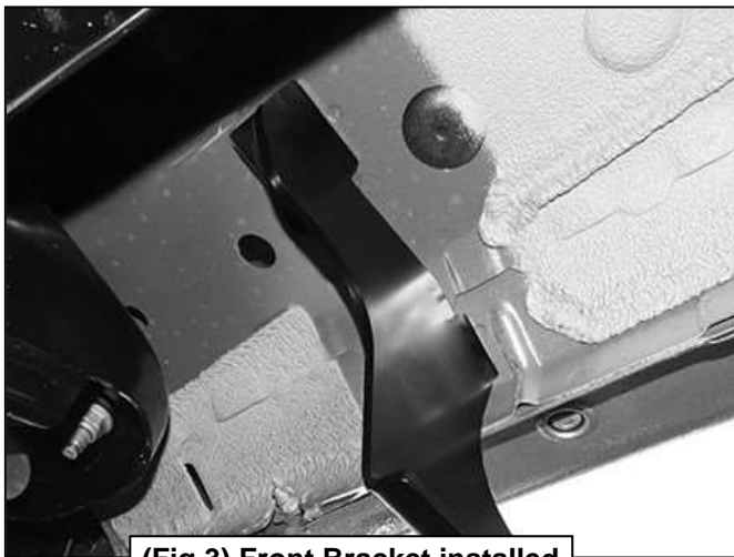
(Fig 3) Front Bracket installed
