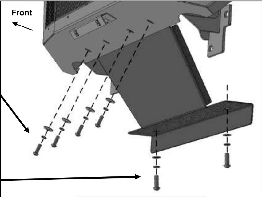
**(Fig 2) Skid Plate fully installed**
