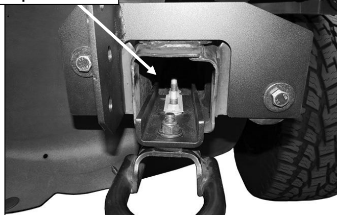
(Fig 9) Tow hook attached to Relocation Bracket
