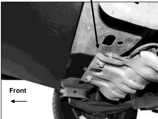
(Fig 7) Reinstall factory STD factory skid plate over MD-1 Skid Plate
