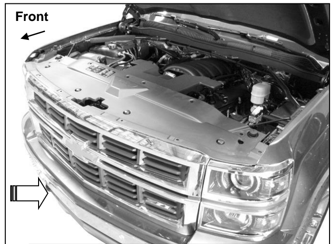
(Fig 2) From behind bumper, release clips along the center and the hardware at the fenders attaching the plastic fascia panel (arrow) to top of bumper. Remove fascia panel to access bumper hardware
