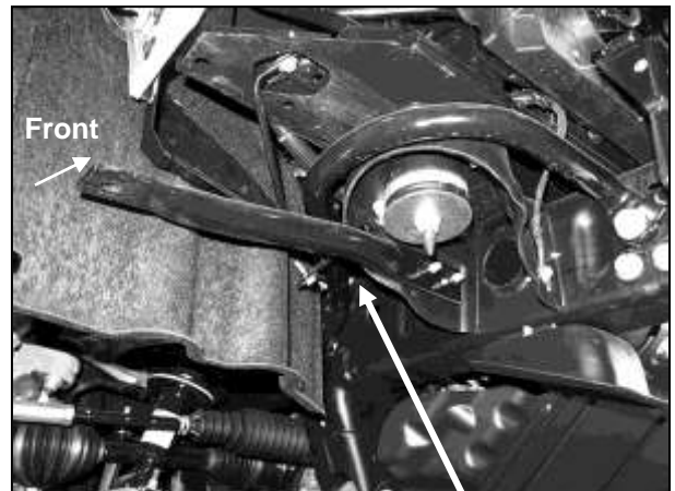
(Fig 4) Remove outer bumper support brackets
