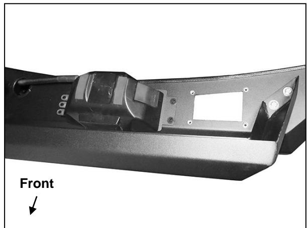
(Fig 31) Attach Relocation Bracket to winch control unit. Attach assembly to top of Bumper
