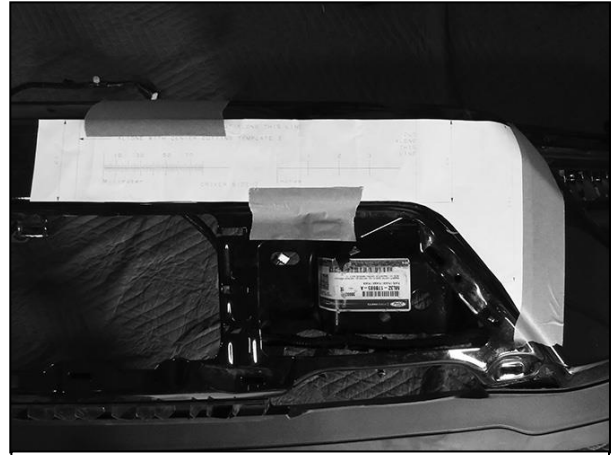
(Fig 8) Place bumper Cut Template onto front bumper. Trace outline of cut template onto bumper cover. Driver/left side pictured
