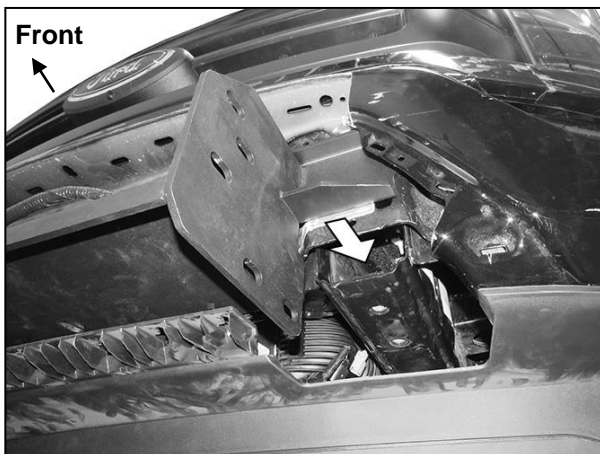
(Fig 22) Models without tow hooks, insert Double Nut Plate into open end of frame (arrow). Reuse the factory hardware to attach the air dam to the bottom of the Winch Tray
