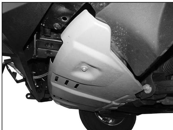
(Fig 31) Reuse factory hardware to reinstall skid plate or splash guard
