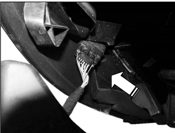
(Fig 5) Pull the bumper out slightly and unplug the outer wire harness
