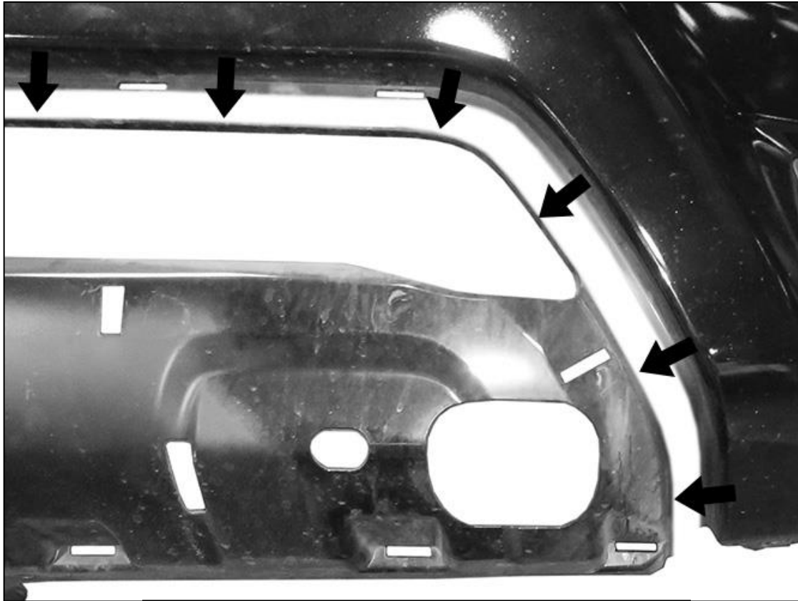
(Fig 13) Use a sharp knife or hacksaw blade to cut along cut line and remove lower section (diver/left side pictured)
