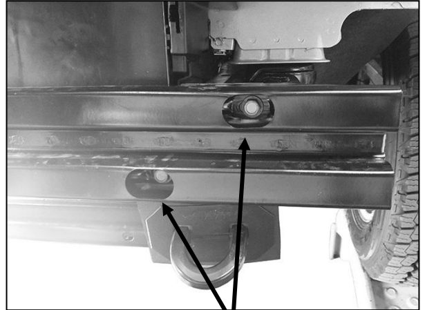
(Fig 9) Remove (2) hex bolts (arrows) from driver/left side of impact bumper
