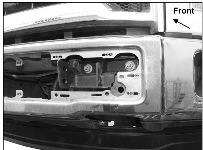
(Fig 4) Driver/left Frame Bracket installed
