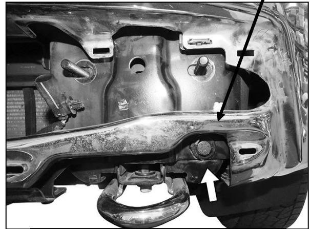
(Fig 9) Reinstall factory bumper. Use included 12mm hardware to attach bottom of bumper (arrow)
