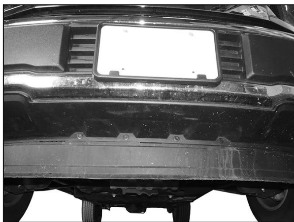
(Fig 1) Remove license plate from Bumper
