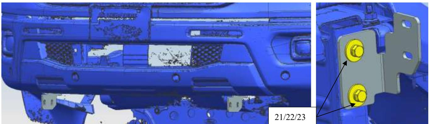
Step 4: Place the brace brackets through the bottom of the plastic grille guard and then fixed with the original standard parts. The left and right side installation are consistent.
