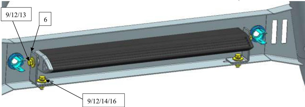
Step 3: Install the bracket L/R on the girder with standard parts. The left and right side installation are consistent.
