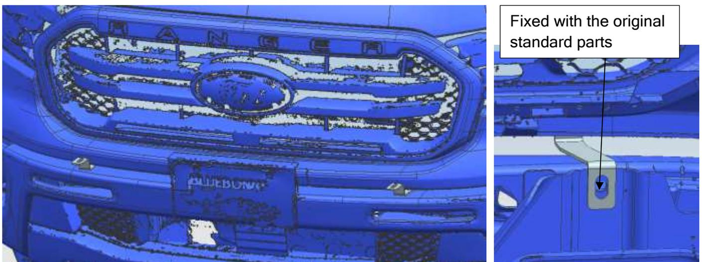
Step 5: Find out the inner radar plastic bracket from the front runner (or from the radar bracket). Then fasten the original radar on the front runner as the below shown. In addition, install the radar brackets on the front runner after the radar brackets are installed with below standard parts.
