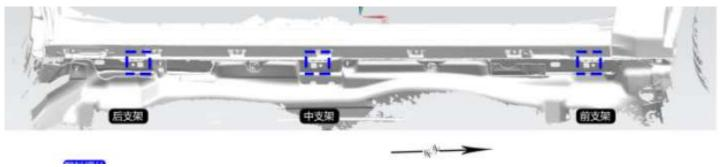
Step 2. : Insert the ① special plate into the square hole, align the screw with the round hole, fix the positioning hole with the plastic screw, and fix the ② special plate to prevent it from falling off. The front the mounting bracket is fixed with M8\*12 flange bolts, and the rear end is fixed with M8\*20 flange bolts.
