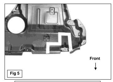
Hold the plastic splash guard up to the bottom of the brackets. Trace location of brackets onto the inside of the splash guard. Picture used for example only
