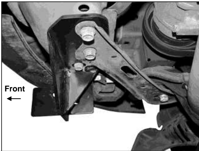
(Fig 3) Passenger/right Mounting Bracket installed
