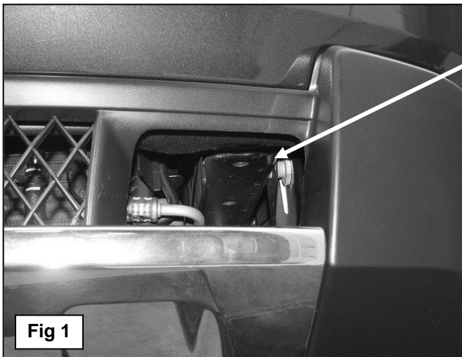
2011-13 Tow hook mounting location pictured through opening in front bumper cover. Remove tow hook if equipped
