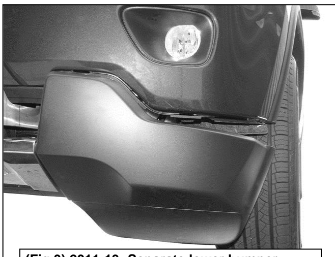
(Fig 3) 2011-13: Separate lower bumper cover from upper bumper cover at ends only
