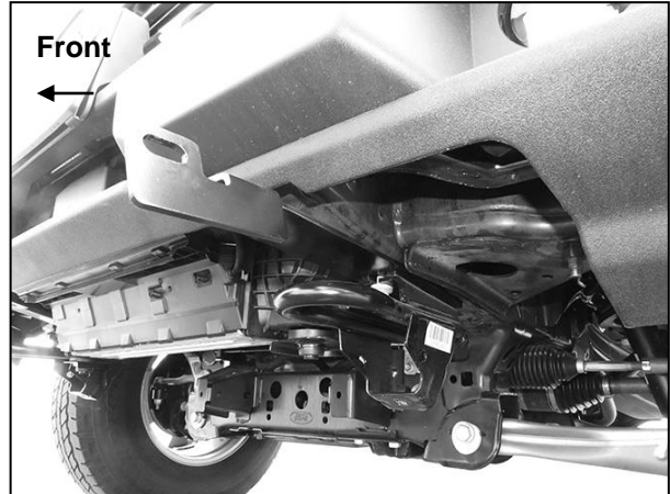
(Fig 4) Models with plastic bumper cover, insert driver/left Support Bracket between frame and tow hook
