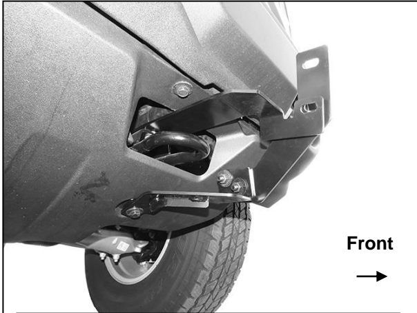
(Fig 11) Driver/left side Brackets installed
