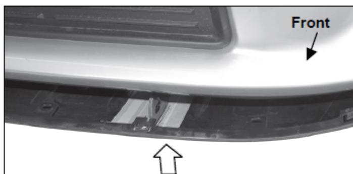
(Fig 9 ) Hold the splash guard up to the bottom of the brackets and mark location for cutting to clear brackets. Cut only what is needed to insert bracket through the splash guard.
