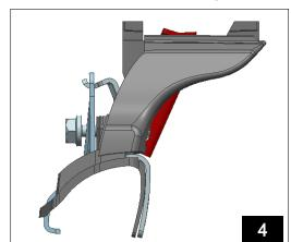
Step 2: Refer to the picture below and assemble brackets (2) to cross bar (1);
