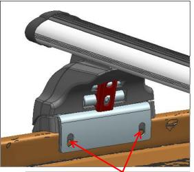
Mark positions and drill holes with size  $\varphi$  4.8.
