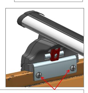
6 Fasten the brackets with self-tapping screw – 8 locations in total
