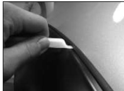
Using flat end of Edge Trim Tool, seat edge trim against flare by inserting straight end between edge trim and flare at one end. Next, slide around entire edge to the other end.
