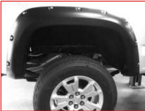
Holding flare in position, start five supplied screws (SW1-0056) into one forward and two rearward mounting holes.
