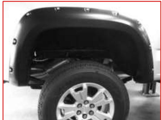
Fully tighten all screws, starting through the top center hole working outward. Use awl to align clip with mounting holes.
