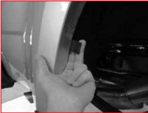
Wrap five supplied tabs around inner lip of sheet metal over the marked locations.
