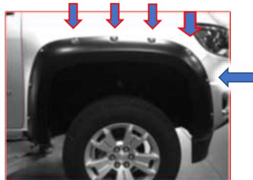
Hold flare in place and start the five Pan Head Screws into the top three and front two holes. Do not fully tighten.
