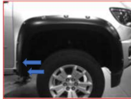
Start two supplied screws into the two bottom rear mounting locations. Fully tighten all screws.
