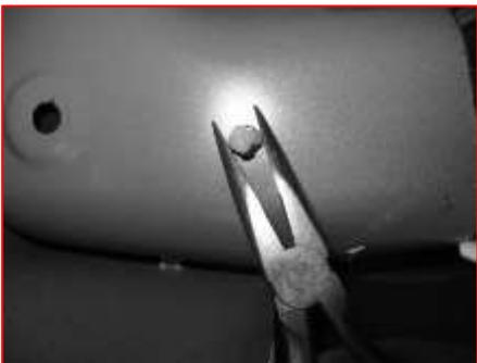
Once the factory fasteners have been removed, reach in behind deflector to find white factory retainer. Using pliers, pinch retainer and push towards wheel center, releasing deflector. Discard factory fasteners and deflector.
