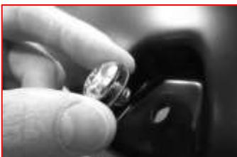
Put each Bolt/Washer combination through a pocket hole in the flare, Bolt head and Washer to the outside.
