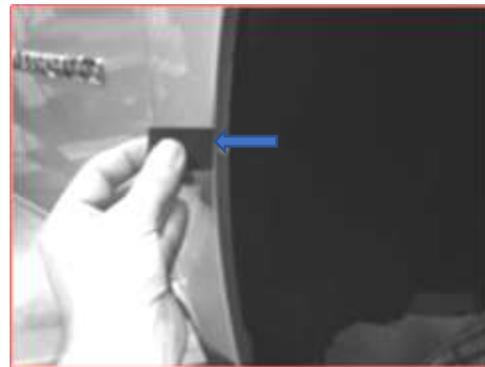
To mark the clip locations, use the flare as a template and hold it in position, use a grease pencil or sharpie to mark sheet metal using hole location as a guide.
