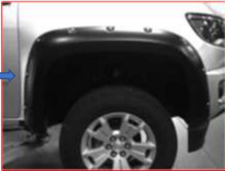
Using an awl, align clip with mounting hole and start one Pan Head screw. Do not tighten.
