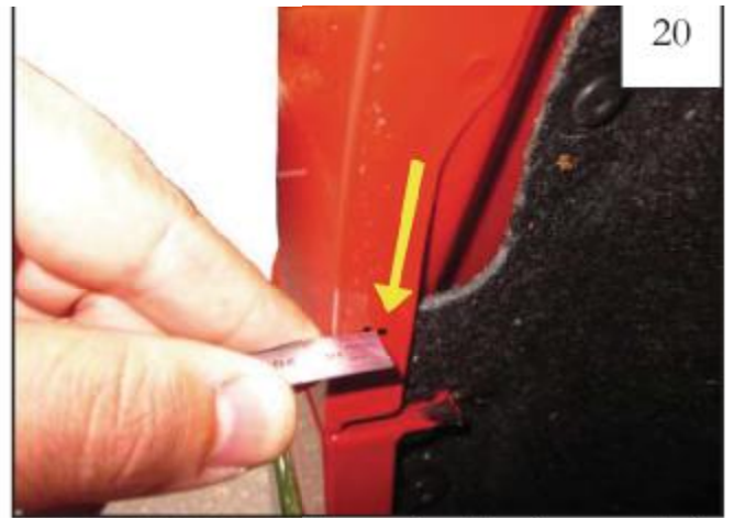
Remove the flare. At the marked locations made in Step 18, measure inward 22mm from the edge of the fender. These are the marks to be drilled.
