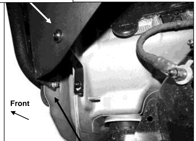
(Fig 15) Attach rear of Fender Liner to "Z" Support Bracket (Fig 7). Attach Liner to back of body panel and fender with the fender hardware or the included (1) 6mm Combo Bolt if long enough
