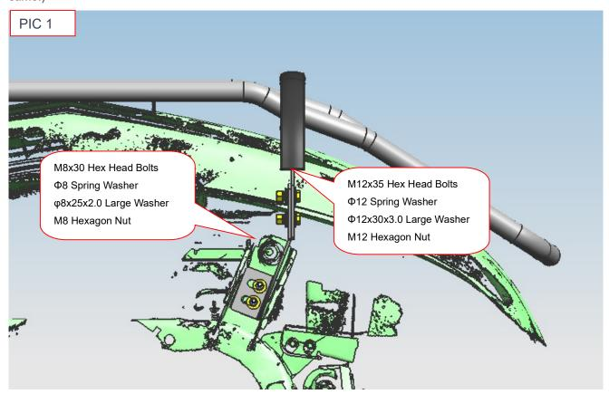
Step 4: Check if all hardware is installed and then fasten all to complete the installation.
