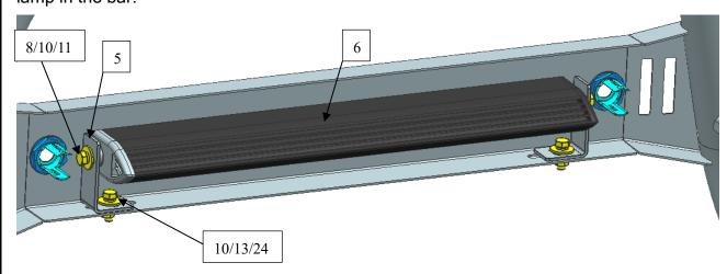
Step 3: Install the brackets L/R in the hole of the trailer. Fasten the brackets with T Double bolt M12 and other standard parts on the girder. The left and right side installation are consistent.
