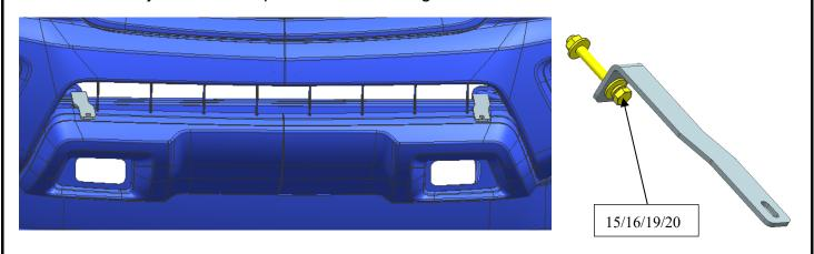
Step 5: Find out the inner radar plastic bracket from the front runner. Then fasten the original radar on the front runner as the below shown.
