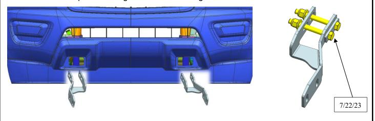
Step 4: Place the support brackets through the plastic grille guard and then fixed in the rear of the collision beam by the standard parts. The left and right side installation are consistent.
