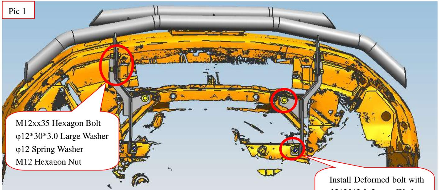
Step 3: Install the bar body on the bracket and adjust the mounting position of the bracket according to the position of the bar body.
