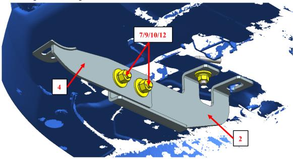
Step 3: Use the standard parts of the front bumper to install the front bumper with mounting bracket 2, consistent on both sides. The following image shows the right side.
