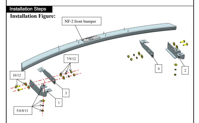
Step 1: Find the two holes on the bottom of the car body where the mounting bracket is installed, and use standard parts for installation. The left and right are consistent, as shown in the figure on the right.
