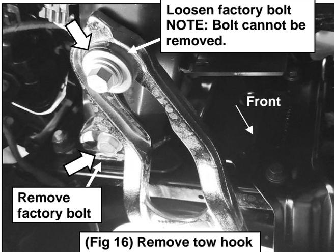
(Fig 16) Remove tow hook (driver/left side pictured)
