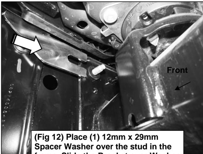
(Fig 12) Place (1) 12mm x 29mm Spacer Washer over the stud in the frame. Slide the Bracket over Washer
