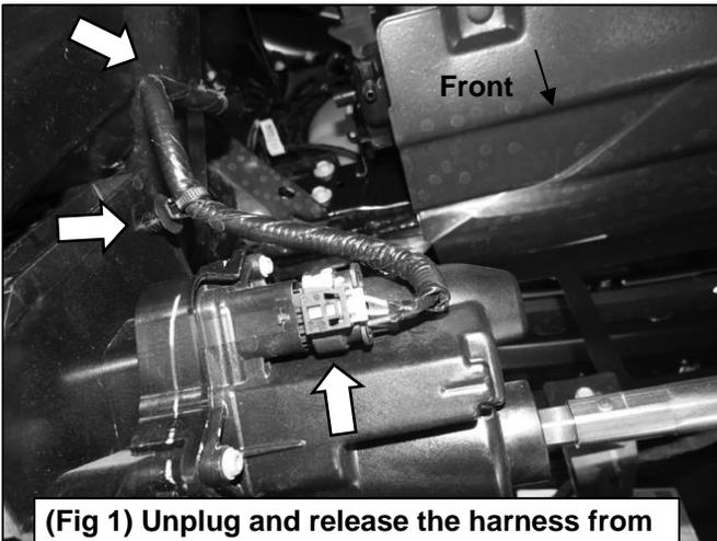
(Fig 1) Unplug and release the harness from the plastic clips to remove active air dam
