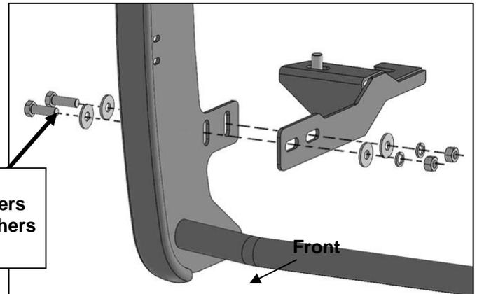
**(Fig 21) Passenger/right side Frame Bracket attached to the inside of the Grille Guard Upright**
