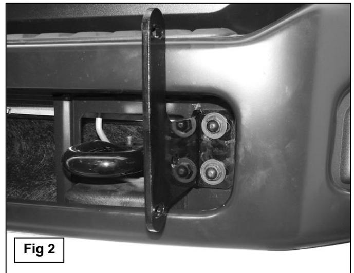
**WARNING!** Do not remove passenger and driver bumper bolts at the same time or bumper may fall. Only remove and install one Frame Mounting Bracket at a time.
