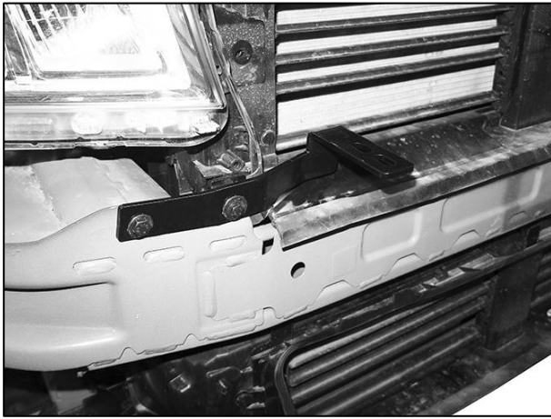
(Fig 14) Passenger/right Top Inner Support Bracket attached to crossbar
