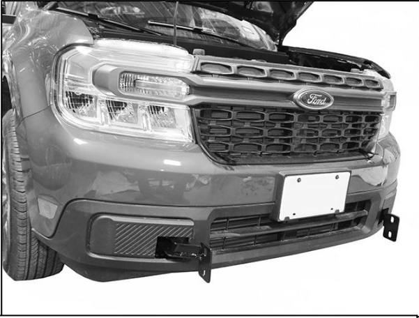
(Fig 20) Temporarily remove the Grille Guard from the Brackets. Reattach the bumper cover after it has been trimmed to clear the Brackets. Plug in wiring harness.
