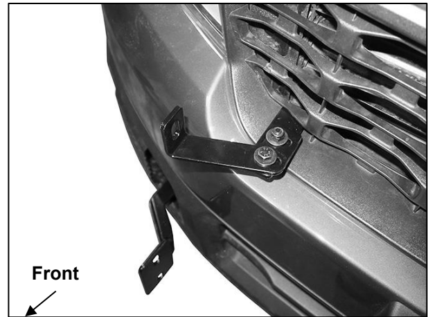
(Fig 21) Reattach the Top Outer Support Brackets (passenger/right side pictured)
