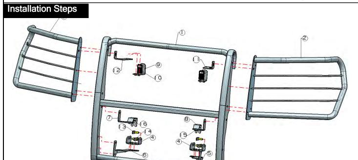
STEP1: Attach Mounting Bracket to Middle Guard, left/right sides installation way are same.
