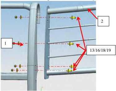
STEP7: Attach Middle Guard to Lower Mounting Bracket and Support Bracket and Upper Support Bracket, left/right sides are installed symmetrically.
