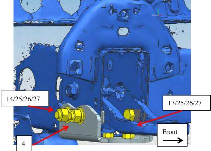
STEP2: Attach Lower Mounting Bracket with Mounting Bracket, left/right sides are install symmetrically.
