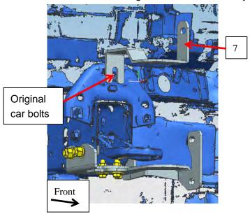
STEP4: Attach Top Support Bracket to the Car, left/right sides installation way are same.
