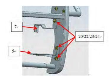
STEP 8: Adjust the gap between Middle Guard and Car body, tighten all hardware.
