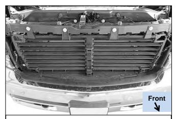
(4-2) Remove screws attaching grille and carefully pull grille straight out to remove grille
