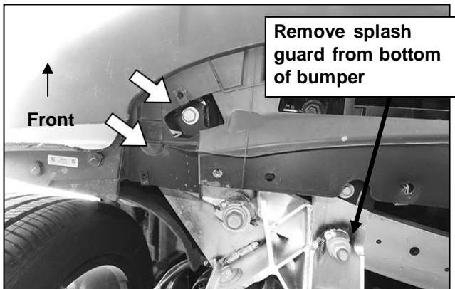
(Fig 5) Remove splash guard. Locate the large 21mm (under plastic cover) and small 16mm (visible) hex bolts (arrows)
