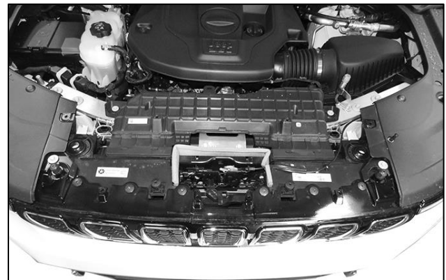
(Fig 6) Remove the hardware connecting the top of the grille to the crossbar. Gently pry the grille and bumper from the vehicle
