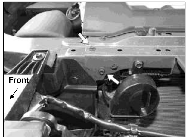
(Fig 10) Remove the (2) hex bolts from the passenger/right side of the radiator core support (arrows)
