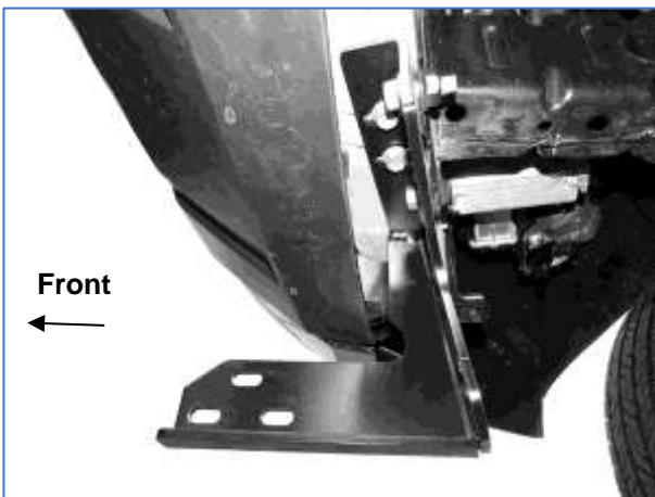
(Fig 3) Passenger/right Frame Mounting Bracket installed
